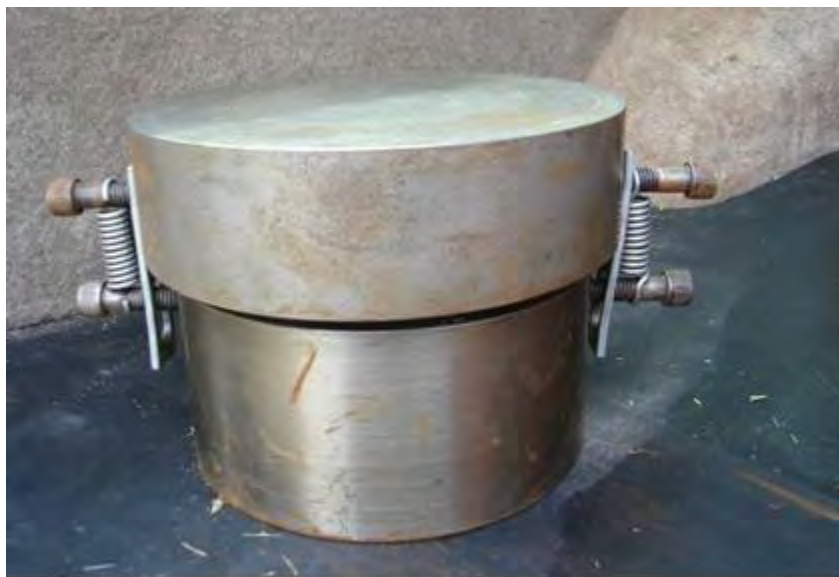
PHOTO 9: Loading plates with ball and matching cup.
