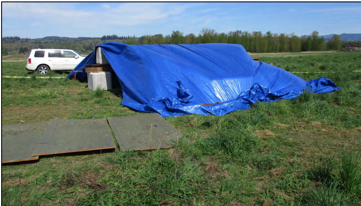
PHOTO 8: Typical compression load test reaction frame setup after covering with tarp.
