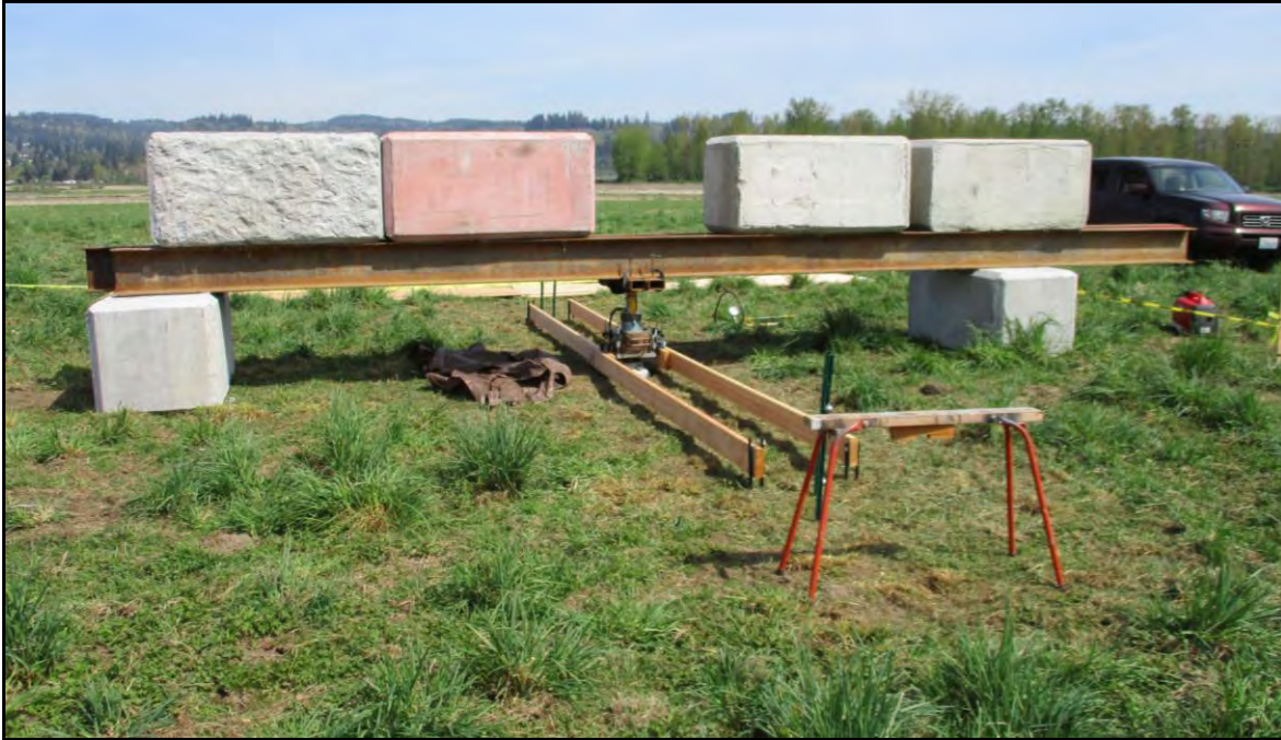
PHOTO 7: Typical compression load test reaction frame setup.
