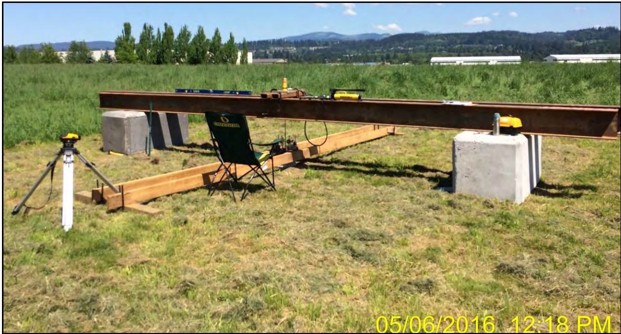
PHOTO 7: Typical uplift load test reaction frame setup.
