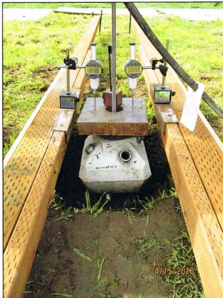
PHOTO 8: Typical uplift load test setup.
